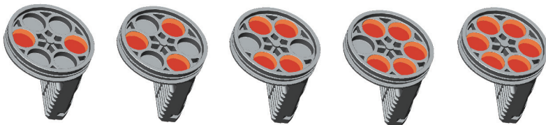
Shown are the spring locations per piston.
