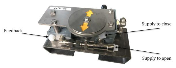
8. Make sure all tube connections are tightened and apply airpressure to the system. Use dedicated leakspray to find possible leaks, operate the actuator and perform another leaktest.
