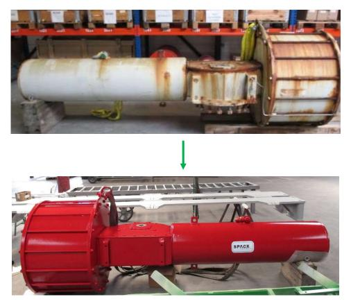
All actuators will be functionally and leak tested, and if required we can include for a torque test as well. A standard warranty on the repair/overhaul is 12 months.
