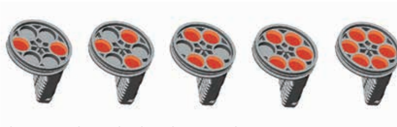
Shown are the spring locations per piston.
