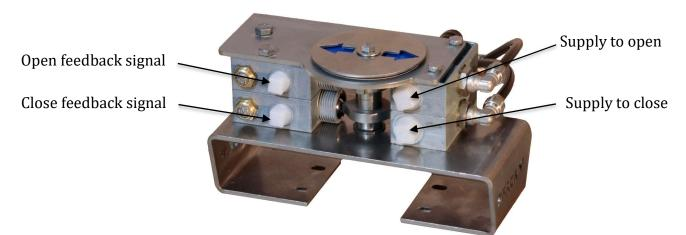
8. Make sure all tube connections are tightened and apply airpressure to the system. Use dedicated leakspray to find possible leaks, operate the actuator and perform another leaktest. Your DA-D-D2 position feedback module is now ready for testing.
