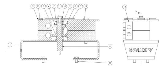
Part #1 and #6 may differ, with ordering spare parts the relevant NAMUR size has to be detailed.
