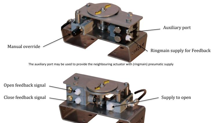
8. Make sure all tube connections are tightened and apply airpressure to the system. Use dedicated leakspray to find possible leaks, operate the actuator and perform another leaktest. Your SR-D-D2 position feedback module is now ready for testing.
